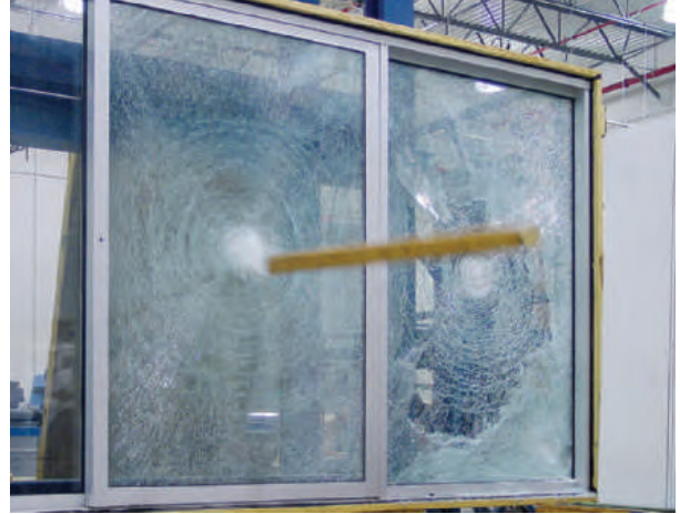
All YKK AP ProTek™ window & sliding door systems are fully tested for Large & Small Missile Impacts compliant with South Florida Building Code Test Protocols TAS 201, TAS 203, and ASTM E 1886 & 1996.
