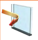
In summer, Low E glass keeps hot air out and cool air in.
