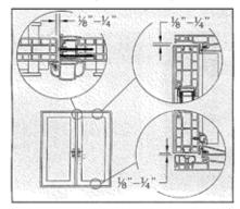
To increase clearance at the bottom of panel (Arrow A), shim at the specified place (Arrow B). To decrease clearance at the bottom of panel (Arrow A), shim at the specified place (Arrow C).
